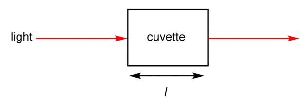
Figure 1: Light absorbed by sample in a cuvetter
